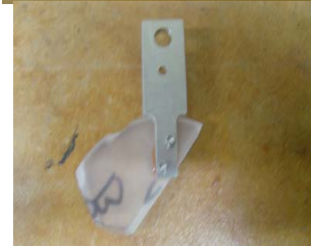
Figure 24: Bonded flexure pull-test fixture. The fixture was used to test shear strength (left) and tensile strength (right) of flexure pads bonded to lens material samples.
